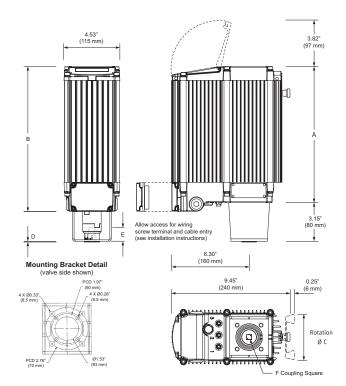
G12 is a 310 in.lb torque: 24vDC 3.5 Amp. G13 is a 885 in.lb torque: 24vDC 5.0 Amp.
