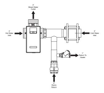
\*DRV50R is a DRV80 supplied with 3" x 2" Bushings at the hot inlet. 2" recirculation manifold and outlet.
